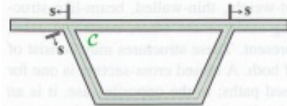
Fig. 8.3. Thin-walled beam with open and closed components.
