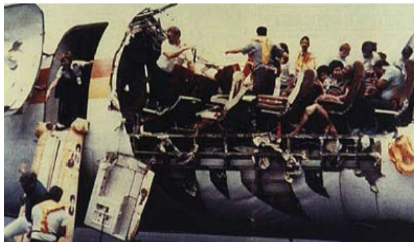
Fig.1.4 Aloha Airlines Flight 243, Boeing 737-200, April 28 1988, Honolulu, Hawaii (undetected cracks in fuselage skin, corrosion in the joint as a result of disbonding)
