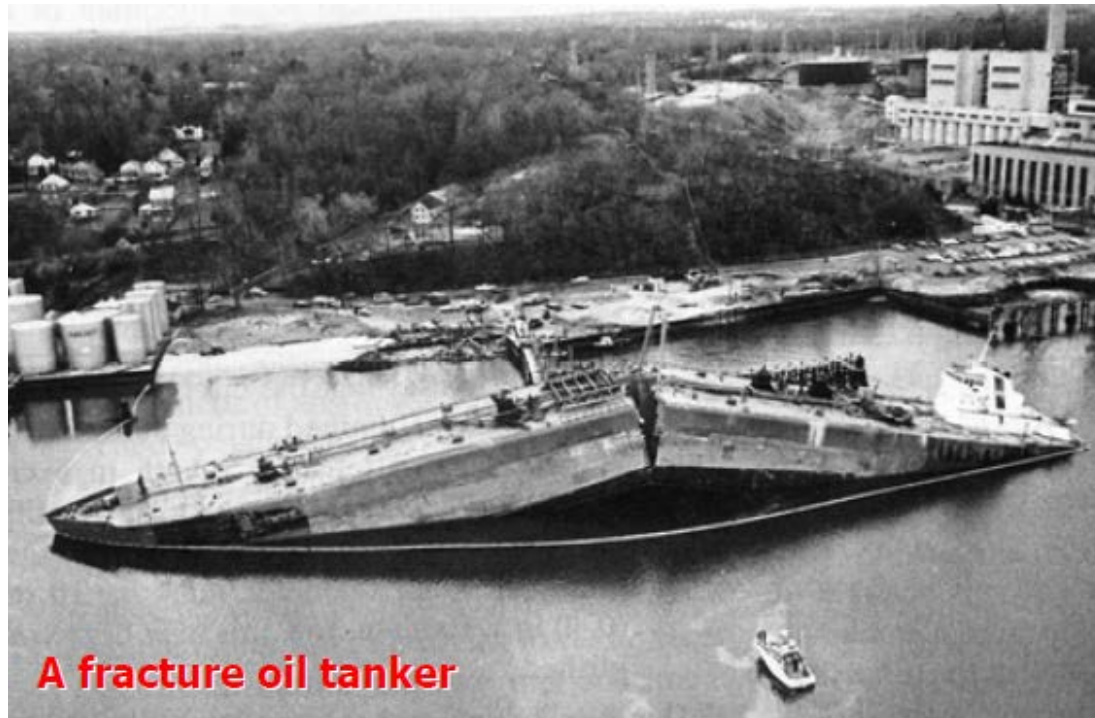
Fig.1.2 An oil tanker that fractured in a brittle manner
