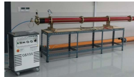
Test bed for OTDR verification test
