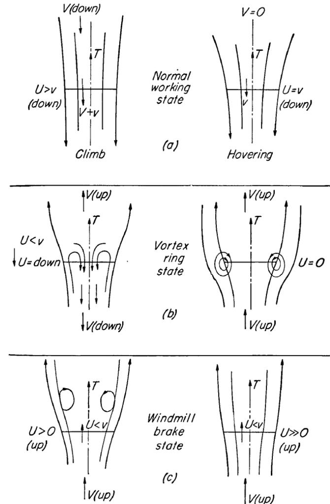
Fig. 6-6 Flow states of an airscrew.
