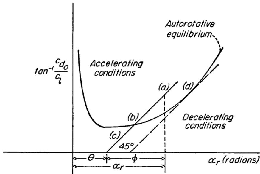
Fig. 6-3 Autorotation diagram for investigating equilibrium conditions at a blade element.
