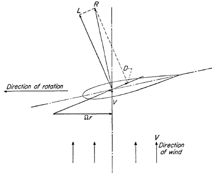
Fig. 6-1 Forces acting on a windmilling blade element.
