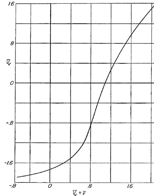
Fig. 6-9 Empirical curve for calculating vertical-descent velocities.
