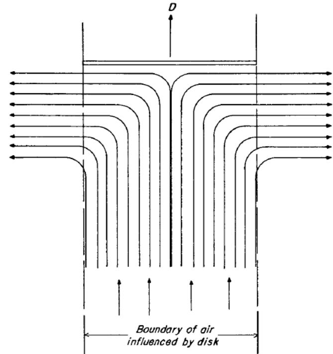
Fig. 6-10 Flow picture for calculating drag of disk by Newton's law.
