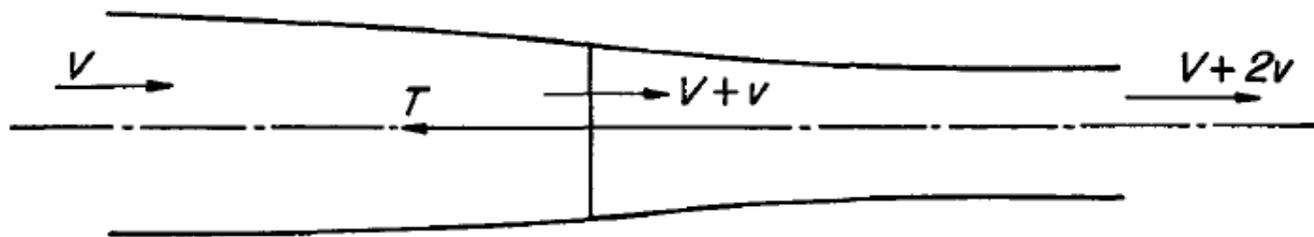
**Fig. 6-5** Slipstream of an aircrew as derived from momentum considerations.
