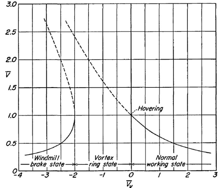
Fig. 6-7 Theoretical induced-velocity parameter. (Dashed lines indicate region wherein momentum concepts do not apply.)
