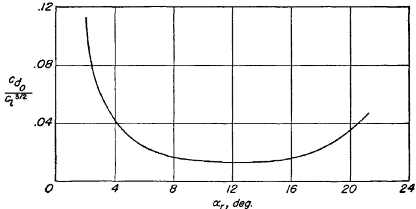
Fig. 6-4 Section characteristics of a practical-construction NACA 23012 airfoil.
