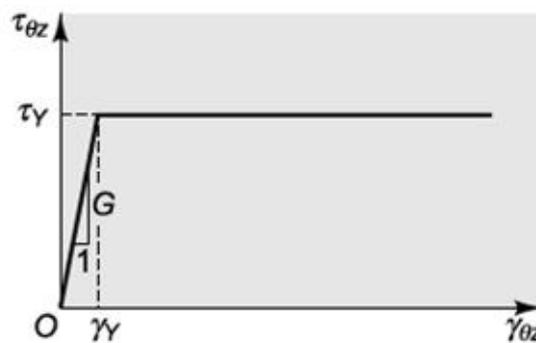
**Fig. 6.19** Shear-stress–shear-strain curve for elastic-perfectly plastic material
