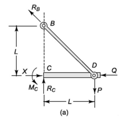
The total strain energy in this case 1s due to longitudinal and bending loading in *CD* and to longitudinal loading in *BD*,
