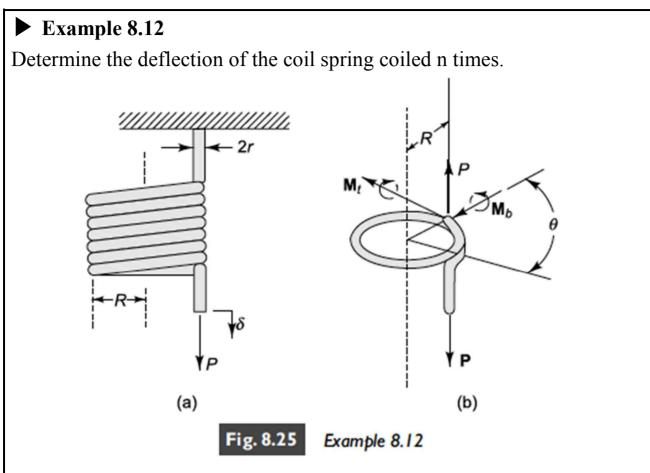
At each section of the spring, the wire carries a transverse shear force P, a twisting moment  $M_t$ , and a bending moment  $M_b$ , as indicated in Fig 8.25b. By applying the equilibrium requirements to this free body, we find
