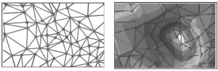
Figure 8.5: An example of topological structure in TIN model.
