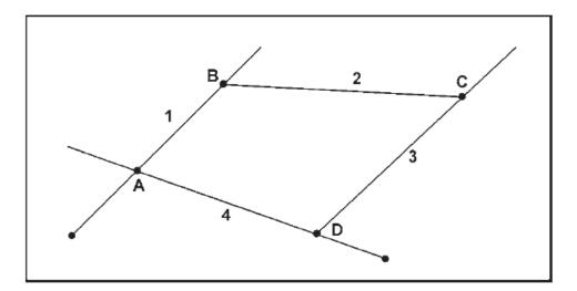
Figure 8.8: A road network splits into links and nodes, here link is a line without logical intermediate intersection and a node is an intersection point where two or more links meet or a start/end point.
