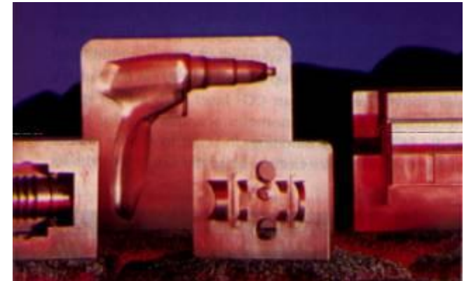
Core and cavity sets produced by RapidTool ™
