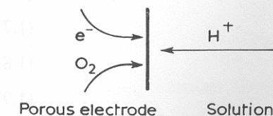
(g) Gas reduction in porous gas diffusion electrode,
