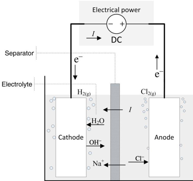
**Figure 1.4** Electrochemical cell for the chlor-alkali process.
