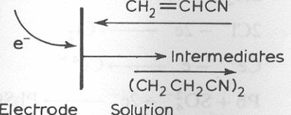
(h) Electron transfer with coupled chemistry,
