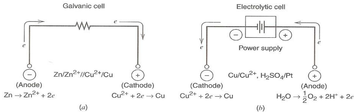
Figure 1.3.1 (a) Galvanic and (b) electrolytic cells.
