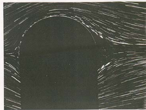
25. Sphere at R=9.8 . Here too, with wall effects negligible, the streamline pattern is distinctly asymmetric, in contrast to the creeping flow of figure 8. The fluid is evidently moving very slowly at the rear, making it difficult to estimate the onset of separation. The flow is presumably attached here, because separation is believed to begin above R=20 . Streamlines are shown by magnesium cuttings illuminated in water. Photograph by Madeleine Constanceau and Michele Poyard
