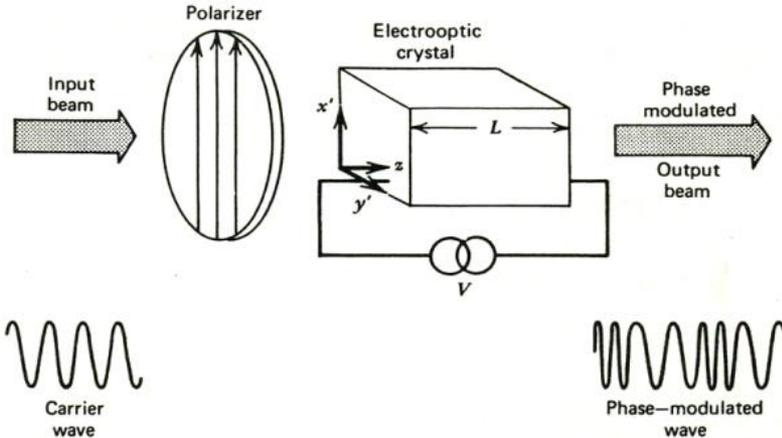
$$E_{out} = A \cos \left[ \omega t - \frac{\omega}{c} (n_o + C_L E_m \sin \omega_m t) L \right]$$
