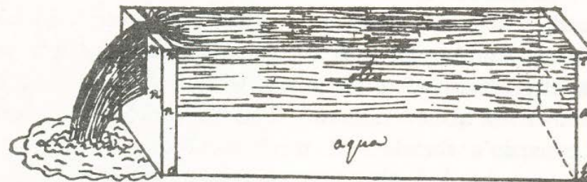
Sketch by Leonardo of flow over a contracted weir.
