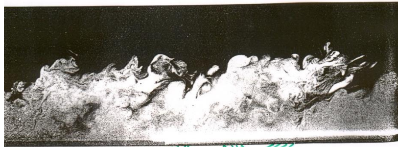
158. Turbulent boundary layer on a wall. A fog of tiny oil droplets is introduced into the laminar boundary layer on the test-section floor of a wind tunnel, and the layer then tripped to become turbulent. A vertical sheet of light
