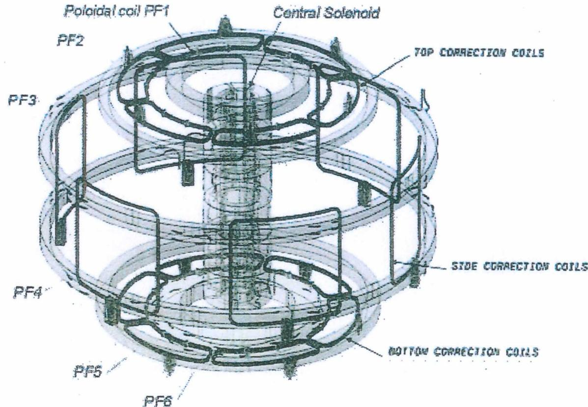
Fig. 1. Layout of correction coils system.
