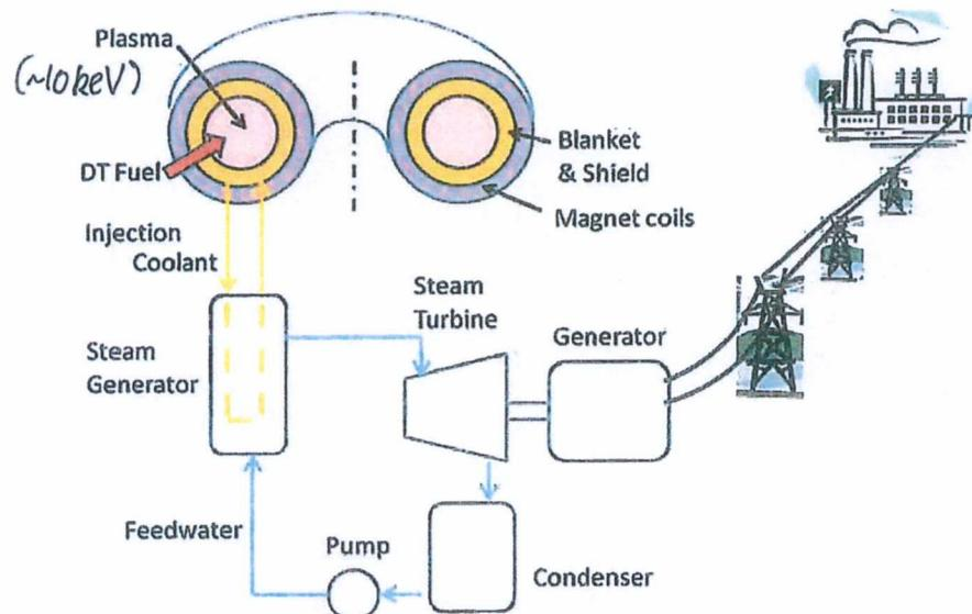
Fig. 1.4 Simplified cutaway view of a fusion reactor connected to a Rankine cycle (steam turbine cycle) to generate electricity. DT means "deuterium-tritium"
