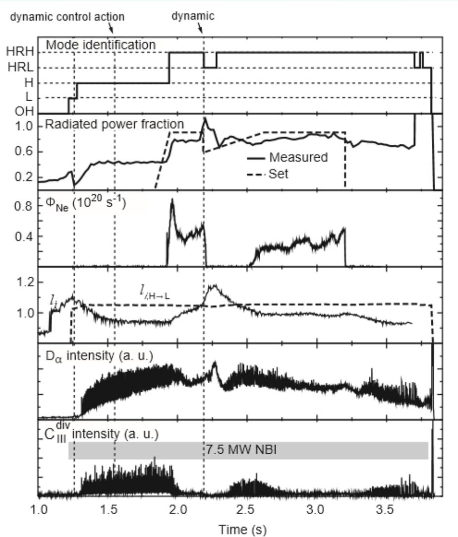
Disruption avoidance in ASDEX-U : upon detection of loss of HRH mode (high radiation H-mode)
