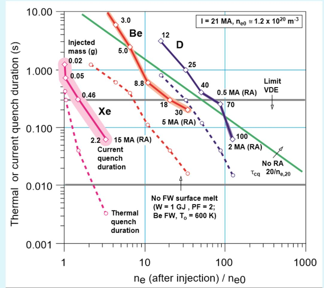
Thermal and current quench durations for fast plasma shutdown in ITER with various quantities (masses in g) and species of injected impurity
