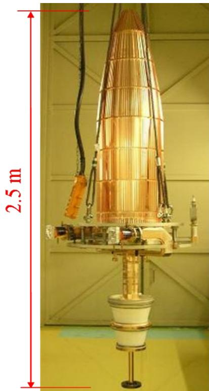
500 kW klystron for
