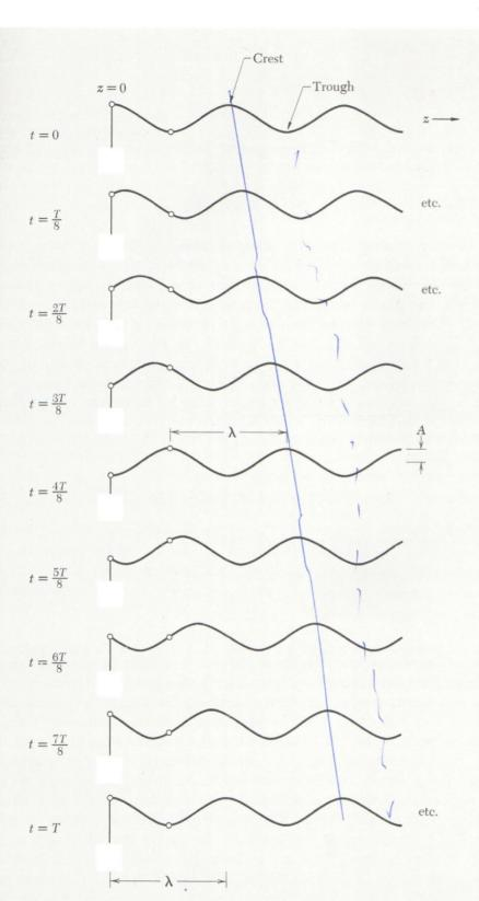
Fig. 4.1 Driving force at z=0 describes harmonic motion of period T. Sinusoidal traveling wave propagates in +z direction. The wavelength is  $\lambda$ . The phase velocity is  $\lambda/T=\omega/k=\lambda\nu$ . Every point on the string undergoes the same harmonic motion as that at z=0, but at a later time.
