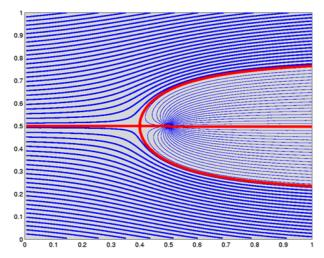
We can mimic a complex flow with proper distributions of sources/sinks, vortices, doublets, and etc.
