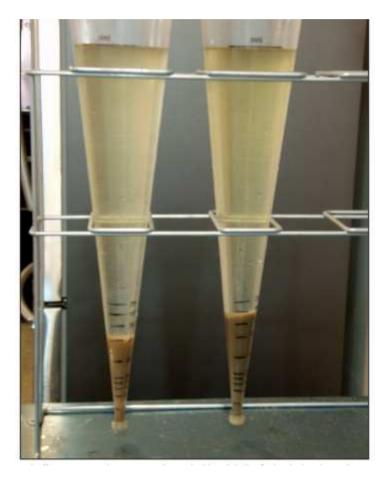
Add 1L in Inhoff cone, wait for 1 hr for settling & record the volume of the thick, bottom layer (reported as mL/L)
