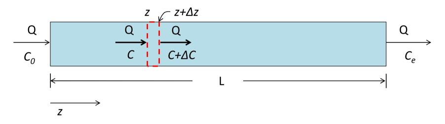
We may take CV as a thin plate perpendicular to the flow at z=z with a dimension of  $\Delta z$  in z dir.
