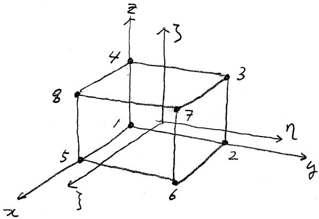
$$\left\{ \begin{array}{l} u = f_1 u_1 + f_2 u_2 + f_3 u_3 + f_4 u_4 + \dots + f_8 u_8 = \sum_i f_i u_i \\ v = \sum_i f_i v_i \\ w = \sum_i f_i w_i \\ x = \sum_i f_i x_i \\ y = \sum_i f_i y_i \\ z = \sum_i f_i z_i \end{array} \right.$$
