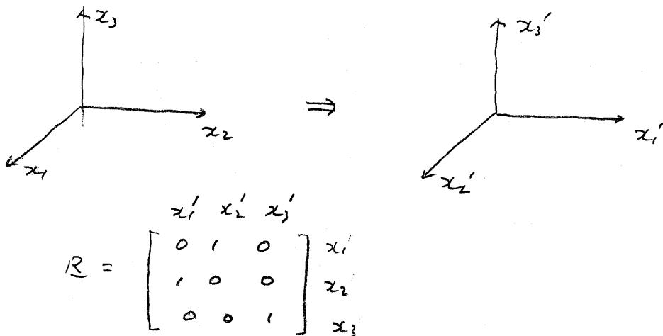
from  $\underline{\underline{C}}' = \underline{\underline{C}}$ ,  $\sigma_{11}' = \sigma_{33}$ ,  $\sigma_{22}' = \sigma_{22}$ ,  $\sigma_{33}' = \sigma_{11}$
