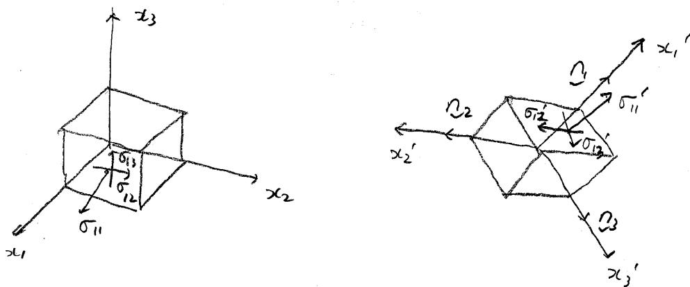
$$\underline{n}_1 = \begin{bmatrix} n_{11} \\ n_{12} \\ n_{13} \end{bmatrix} \quad \underline{n}_2 = \begin{bmatrix} n_{21} \\ n_{22} \\ n_{23} \end{bmatrix} \quad \underline{n}_3 = \begin{bmatrix} n_{31} \\ n_{32} \\ n_{33} \end{bmatrix}$$
