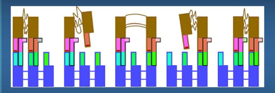
The rise and fall of each foot of the biped is controlled by introducing DNA strands with specific sequences into the solution.
