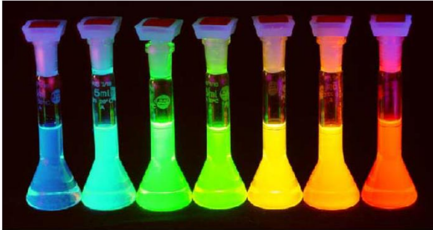
Fluorescence induced by exposure to ultraviolet light in vials containing various sized Cadmium selenide (CdSe) quantum dots.
