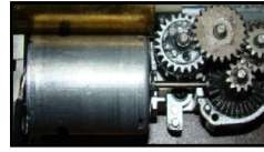
▲ Conventional macro scale actuator (Motor-Gear type)
