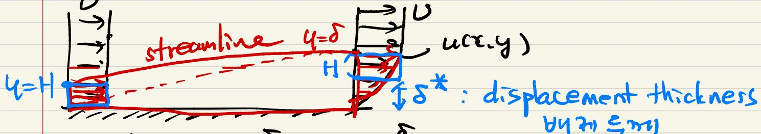
$$\int_0^H U dy = \int_0^\delta u dy = \int_0^\delta (U + u - U) dy$$
