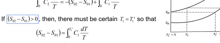
$$(S_{02} - S_{01}) = \int_0^{T_1'} C_1 \frac{dT}{T}$$
