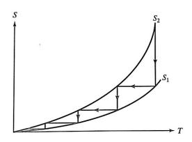
An infinite series of isothermal and adiabatic processes are required to reach absolute zero!
