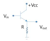
$V_{out}=V_E=V_{in}$ -0.6  $\therefore \Delta V_{out}=\Delta V_{in}$ ; Replica of Input voltage,
