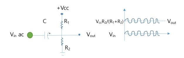
Electrons from  $V_{in}$  ac is getting into the charged capacitor, then overflown (or discharged) electrons are flowing to the voltage divider, riding over the DC offset voltage given by  $R_1$ ,  $R_2$  voltage divider.
