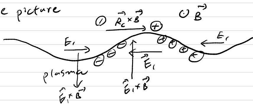
"Interchange" instability (no line bending,  $Q_\perp \gg 1$ ,  $\delta'' \approx 0$ )
