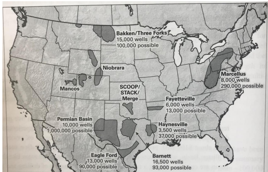
Figure 1.3 Horizontal wells drilled in major unconventional plays in the US as of 2017 and the numbers of wells that could be drilled in the future based on technically recoverable reserves. From Svetlana Ikonnikova, Bureau of Economic Geology, 2017.
