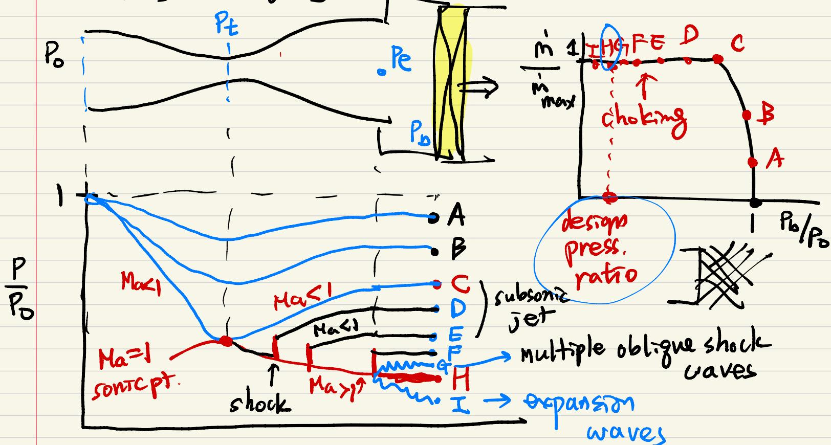
9.7 Compressible duct flow w/ friction
