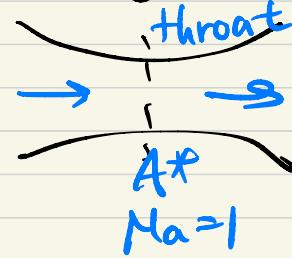
$$\dot{m}_{\max} = \rho^* V^* A^* = P_0 \left( \frac{2}{k+1} \right)^{\frac{1}{k-1}} \sqrt{k R T_0^*} A^*$$
