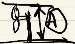
$\mathcal{P}_{\text{available}} = \frac{1}{2} \dot{m} V_1^2 = \frac{1}{2} \rho A V_1^3$
