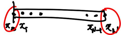
$$\textcircled{2} \quad \left\{ \begin{array}{l} \frac{T_{j+1} - 2T_j + T_{j-1}}{h^2} - d^2 T_j = Q_j \quad j = 1, 2, \dots, N-1 \\ T_0 = 0 \\ T_N = S \end{array} \right. \quad \text{System of algebraic eqs.}$$
