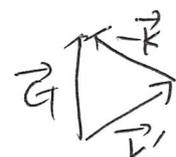
$$\begin{aligned} |\vec{k}' - \vec{k}| &= \sqrt{k^2 + k'^2 - 2\vec{k} \cdot \vec{k}'} \\ &= \sqrt{2k^2 - 2k^2 \cos 2\theta} \\ &= 2k \sin \theta. \end{aligned}$$
