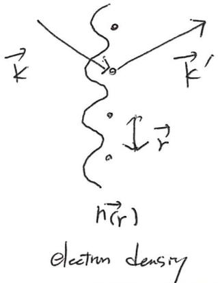
$$\text{Intensity} \propto \left| \int_{\vec{r}} n(\vec{r}) e^{i(\vec{k}-\vec{k}') \cdot \vec{r}} \right|^2$$
