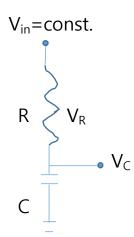
$V_{in}=V_R+V_C=iR+\int idt/C$ , assuming very little current flows into Vc
