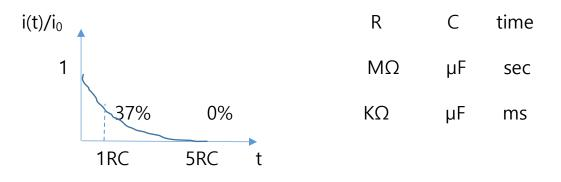
$\therefore$  After 5RC time, no current flows ->Z<sub>C</sub>=Impedance of capacitor= $\infty$
