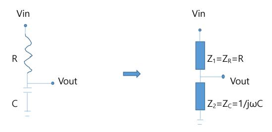
The left RC circuit can be changed as the right circuit of voltage divider, considering that  $Z_R=R$  and  $Z_C=1/j\omega C$
