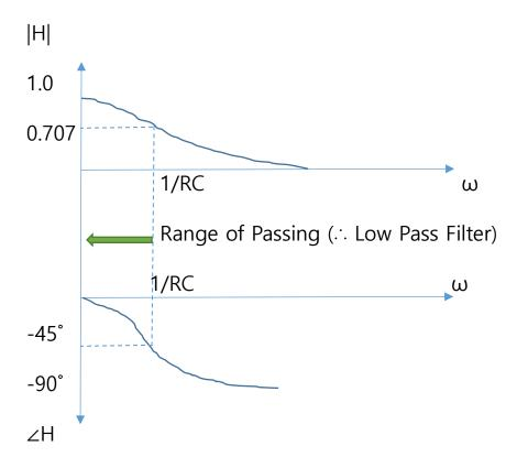
If  $\omega \le 1/RC$  then  $|H| \ge 0.707$  and  $|\angle H| \le 45^\circ$ , and they are acceptable for many engineering application. This circuit effectively can pass the signal of frequency range under 1/RC. Thus it is LPF, Low Pass Filter.
