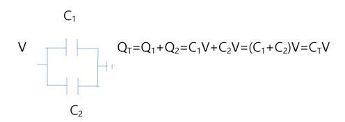
Thus  $C_T = C_1 + C_2 = C_1(1 + C_2/C_1) = 2C$  (if  $C_1 = C_2 = C$ )
