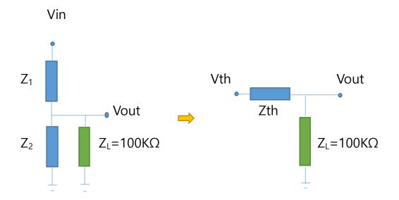
$Zth=Z_1 \parallel Z_2=Z_1Z_2/(Z_1+Z_2)=(R/j\omega C)/(R+1/j\omega C)=R/(1+j\omega RC)$
