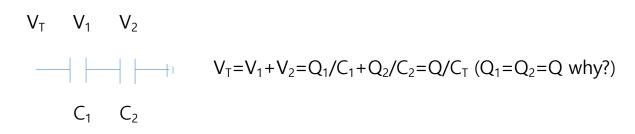
Thus  $1/C_T = 1/C_1 + 1/C_2$ , and  $C_T = C_1C_2/(C_1 + C_2) = C_2/(1 + C_2/C_1)$
