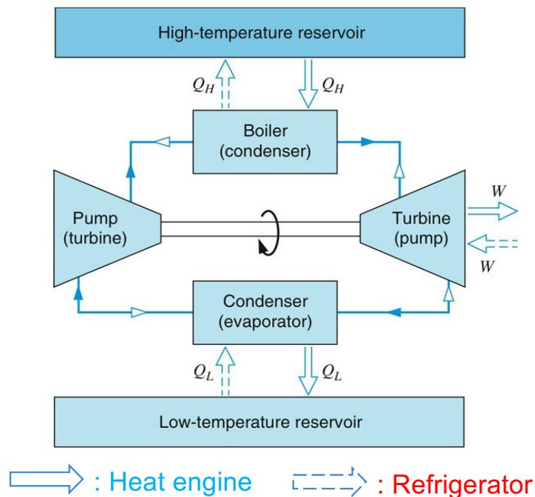
**(Heat engine that operates on Carnot cycle)**
