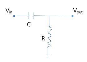
$V_{out}/V_{in}=R/(1/j\omega C+R)=j\omega RC/(1+j\omega RC)$
