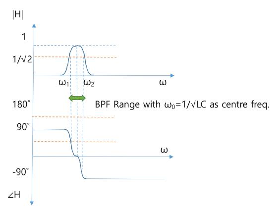
This is the <u>Narrow Band Pass Filter</u> that gives much narrower BPF with centre frequency  $\omega_0=1/\sqrt{LC}$
