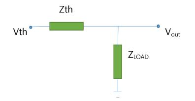
Zth should drive  $Z_{\text{LOAD}}$  and Zth  $\ll Z_{\text{LOAD}}$  is to be satisfied. Therefore,
