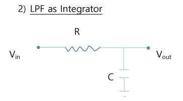
$V_{out}/V_{in}=1/j\omega C/(R+1/j\omega C)=1/(1+j\omega RC)$
