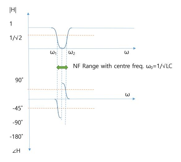
The 3dB frequency  $\omega_1$  and  $\omega_2$  can be evaluated as the freqs that gives the height of  $1/\sqrt{2}$ , by solving the equation
