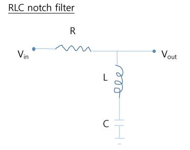
Serial connection of L and C gives the impedance of  $Z_L+Z_C$
