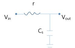
$$V_{out}/V_{in}=1/j\omega C_s/(r+1/j\omega C_s)=1/(1+j\omega rC_s)$$
