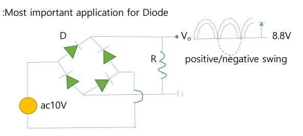
V<sub>o</sub>: Ripple of max 8.8V (=10 – 2xDiode drop)
