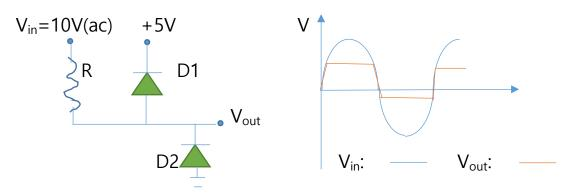
If  $V_{in} \ge 5.6V$  then D1 conducts and  $V_{out} = 5.6V$
