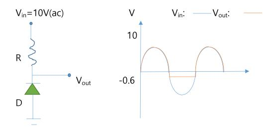
If  $V_{in} > -0.6V$ , then Diode blocks current, thus  $Z_D = \infty$  and  $V_{out}/V_{in} = Z_D/(R+Z_D) = 1 \quad (\because Z_D = \infty) \quad \because V_{out} = V_{in}$ If  $V_{in} \le -0.6V$ , then Diode conducts and  $V_{out} = -0.6V$  (Diode drop)
