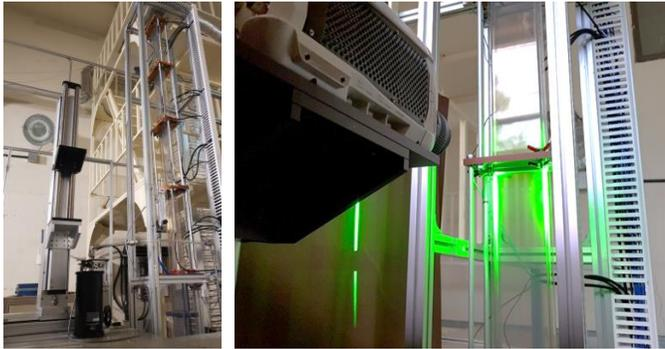
Fabricated liquid film thickness sensor
