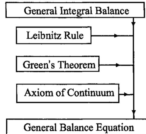
$$\frac{d}{dt} \int_{V_m} F_k dV = \int_{V_m} \left[ \frac{\partial F_k}{\partial t} + \nabla \cdot (v_k F_k) \right] dV$$
