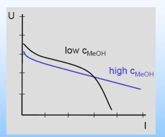
The methanol concentration is always a compromise between cathode and anode impact. It mainly depends on:
