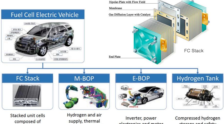
composed of membrane, catalyst, GDL and bipolar plate Hydrogen and air supply, thermal management and water management
