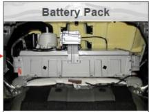
The air cooled NiMH battery pack is packaged in the trunk similar to most Toyota Hybrid vehicles.
