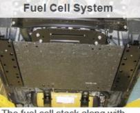
The fuel cell stack along with the boost converter is under the center of the vehicle.
