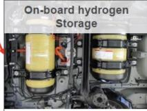
The two hydrogen tanks are under the trunk and the rear passenger seats. These tanks are disabled for the testing.
