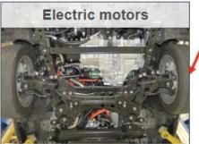
The electric drive motor and the air compressor are packaged in-line between the front wheels.
