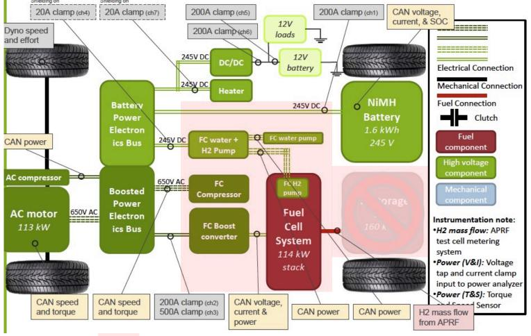
: Fuel cell system, M-BOP and hydrogen tank
