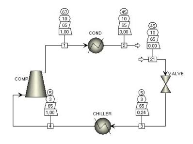
I split the stream 2 into 2 and 21 for better convergence, but closed-loop simulation may work.
