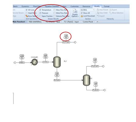
Select the options of Temperature, Pressure, etc. on the "Modify" Tab
