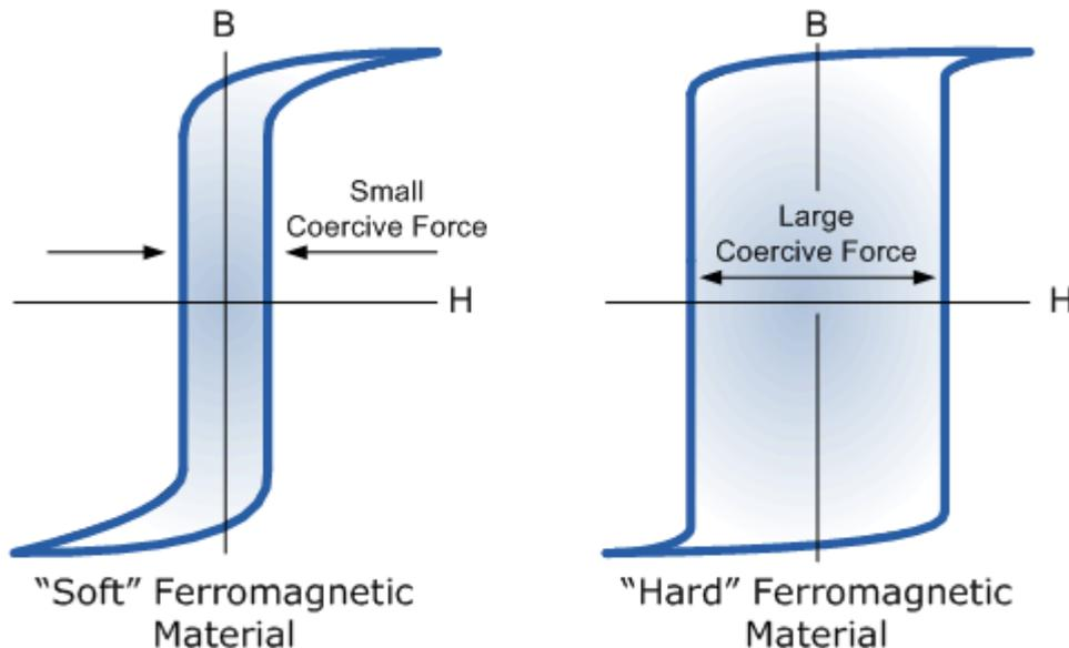
Permanent Magnet Demagnetization Curves
