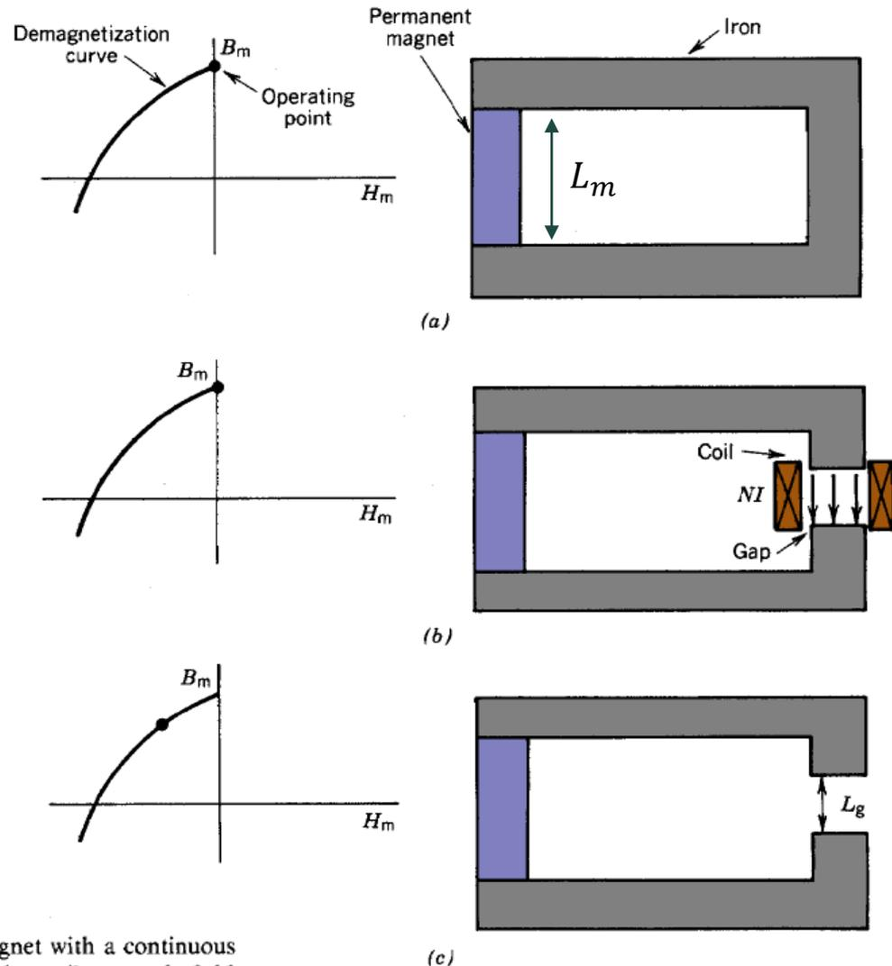
**Figure 5.21** · Operating point of a permanent magnet. (a) Permanent magnet with a continuous iron flux conductor, zero magnetizing force. (b) Addition of an air gap with a coil to supply field energy. (c) Deactivation of the gap coil.
