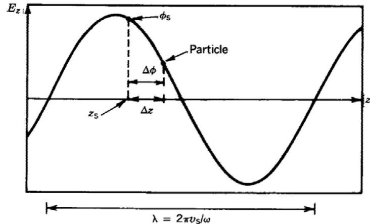
Conditions for having synchronous particles in an accelerator
