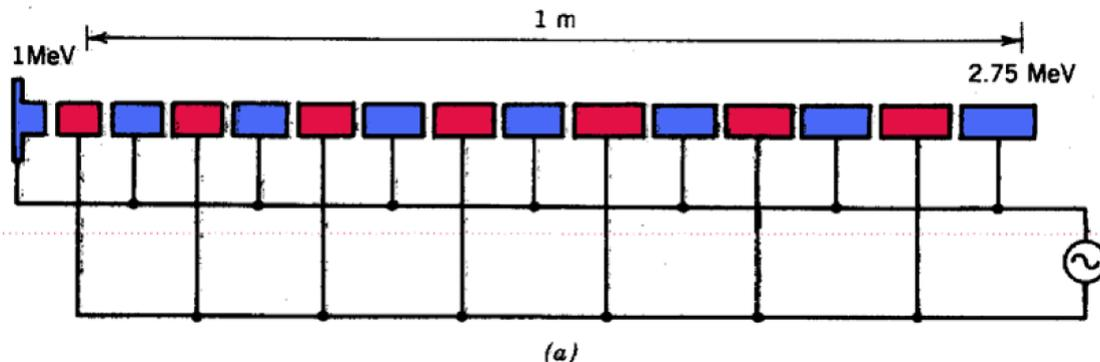
**Figure 14.7** Wideröe linear accelerator for heavy ions. (a) Scale drawing of accelerator with following parameters: Ion species: Cs-137,  $f = 10$  MHz,  $T_i = 1$  MeV,  $V_0 = 100$  kV, and  $\phi_s = 60^\circ$ . (b) Electric fields in acceleration gaps 1 and 2 at ion injection ( $t = 0$ ). (c) Electric fields at time  $t = 1/2f$ , where  $f$  is the rf frequency.
