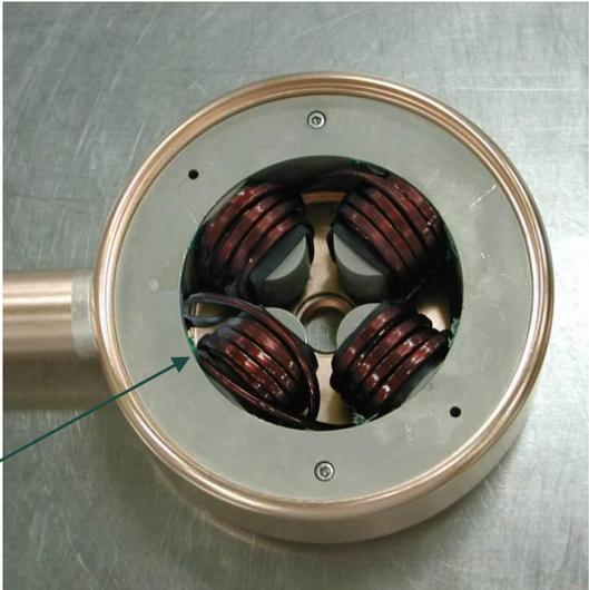
Quadrupole magnet for beam focusing
