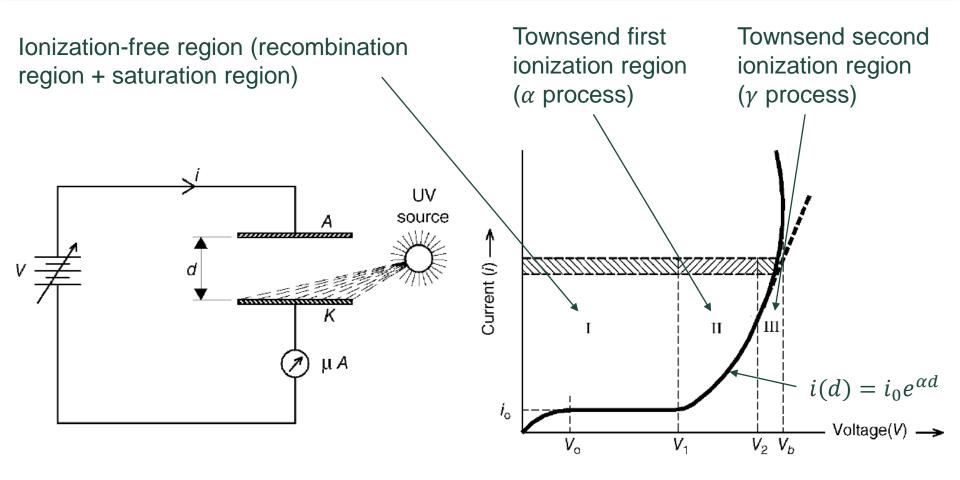
Secondary electron emission by ion impact: when heavy positive ions strike the cathode wall, secondary electrons are released from the cathode material.
