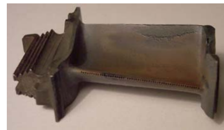
Nickel superalloy in jet engine turbine blade
