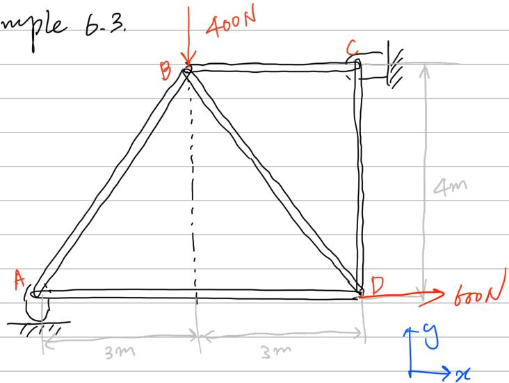
Determine the force in each member of the truss.
