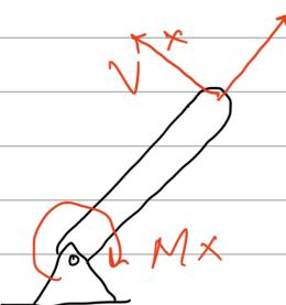
Pin joints cannot handle shear or bending loads.
