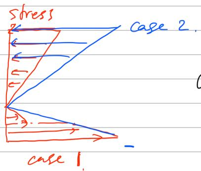
$$\sigma_A = \frac{28.6 \text{ MPa}}{(E_{st}/\epsilon_w)} \\ = 1.71 \text{ MPa}$$
