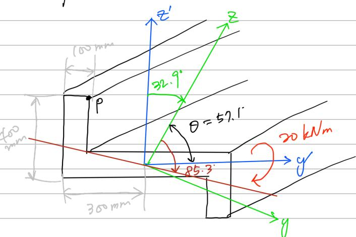
$$\begin{aligned}My &= 20 \cos 32.9^\circ = 16.99 \text{ kN/m} \\Mz &= 20 \sin 32.9^\circ = 10.86 \text{ kN/m}\end{aligned}$$
