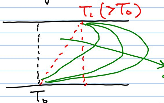
$Br \equiv \frac{\mu U_0^2}{k(T_i - T_0)} \sim \frac{\text{viscous dissipation}}{\text{conduction}}$
