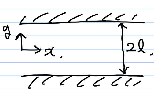
$$\mu \frac{d^2 u}{dy^2} = \frac{dp}{dx}, \quad w/ \text{ @ } y = \pm l, \quad u = 0.$$
