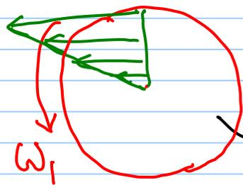
$$v_{\theta}(r) = r \omega_1 ; \text{ Solid-body rotation.}$$
