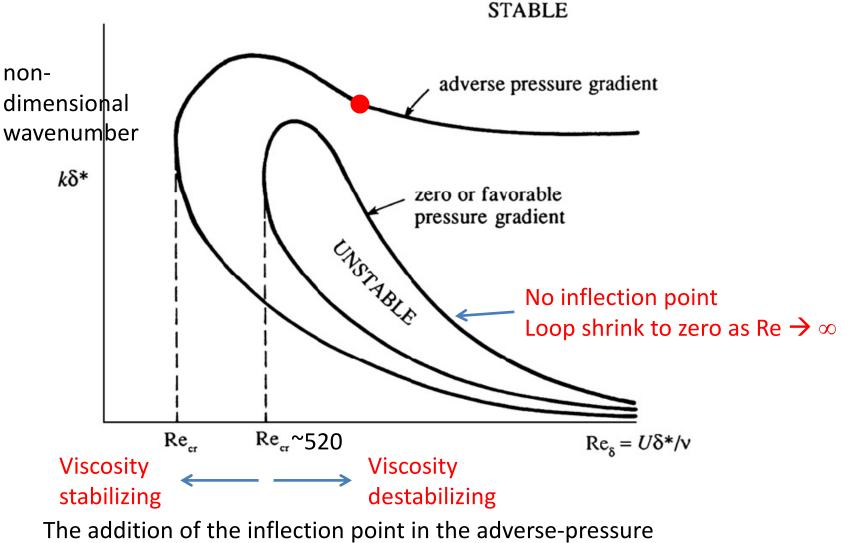
gradient case increases the parametric realm of instability.
