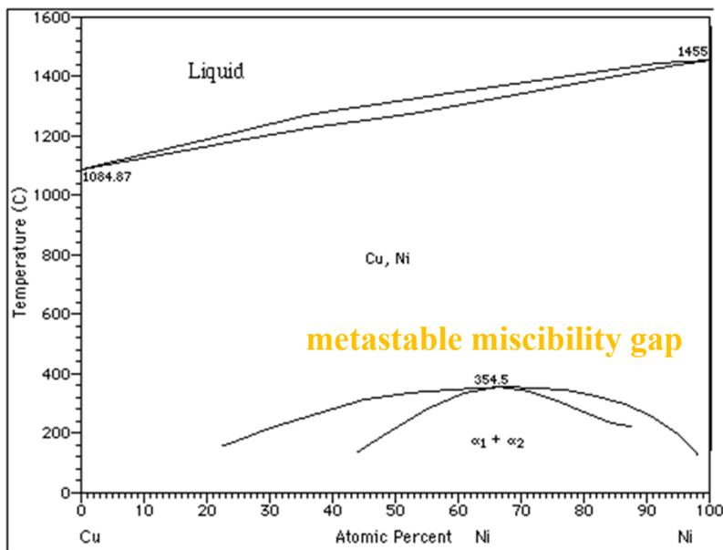
$\Delta H_{mix}^S \gg 0$ : liquid state phase separation (up to two liquid solutions)
