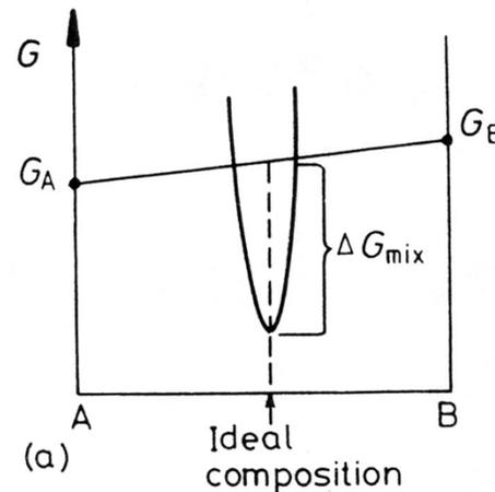
Fig. 1.23 Free energy curves for intermetallic compound with a very narrow stability range, (l stability range.
