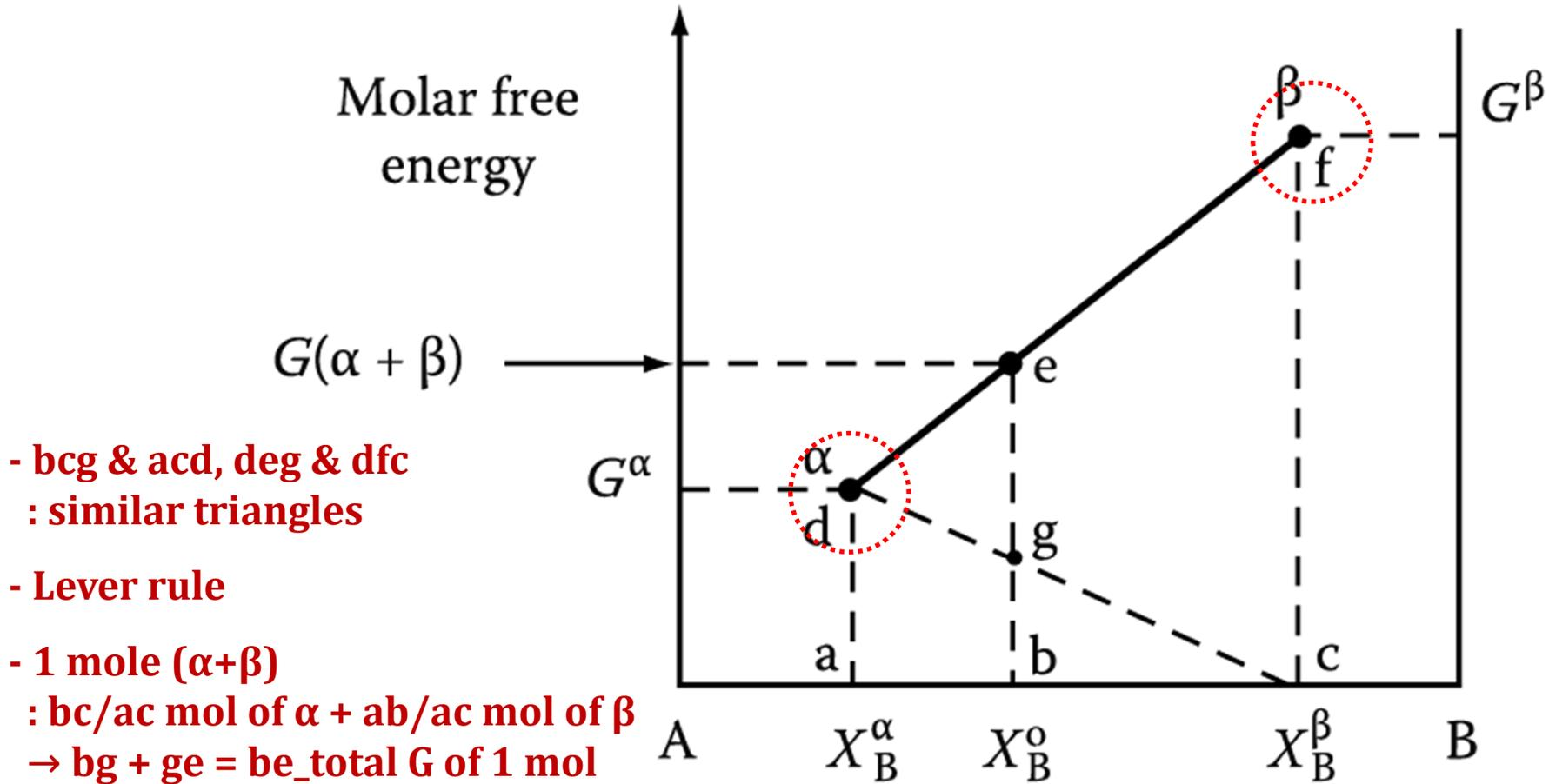
Fig. 1.26 The molar free energy of a two-phase mixture ( $\alpha + \beta$ ) 21
