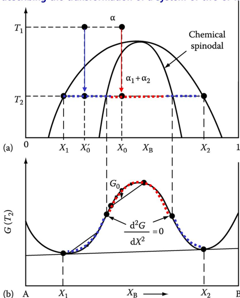
Fig. 5.38 Alloys between the spinodal points are unstable and can decompose into two coherent phases  $\alpha_1$  and  $\alpha_2$  without overcoming an activation energy barrier. Alloys between the coherent miscibility gaps and the spinodal are metastable and can decompose only after nucleation of the other phase.
